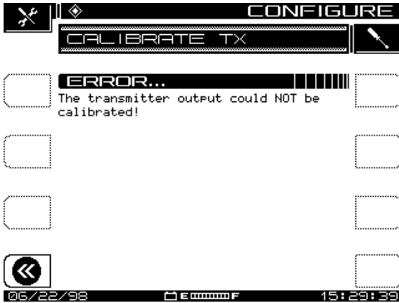
Fig. 2-13 Calibrate Error (Missing Jumper Cable)
